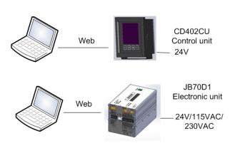
If no switch is available, connect directly to each unit and use its web page to setup. Multirepeaters can be set up directly from the screen.
