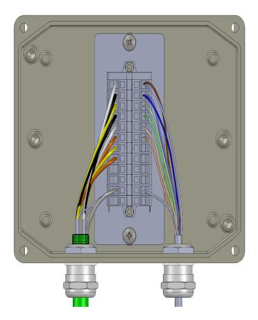
Connect the sensor cable to the Extension cable as shown. All grounds are collected together and connected to the outer ground of the Extension cable. The grounds should **not** be connected to a local ground. If there is no room for the JB12 housing, the cables can be carefully spliced together. Both cables can be cut.
