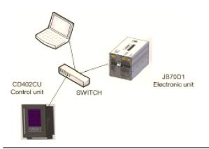
Alternativ 2 Connect CD402 Control unit to JB70D1 via LAN switch
