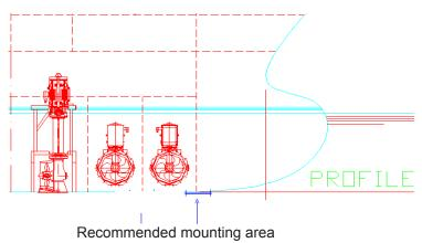
Figure showing the generally best sensor placement in the front region.
