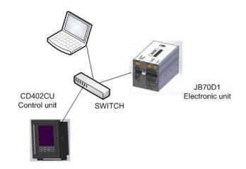
Connect the units together and use SKIPPER service software to find the relevant settings, alternatively address indivdual units using their IP addresses from a web browser
