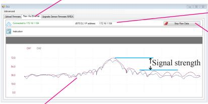
5:The RAW data will be shown as two graphs At 0 knots speed the highest point of graphs will be at at the same point. (Frequency)
