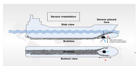
Figure showing placement of a sensor with the individual beams pointing fore and aft.
